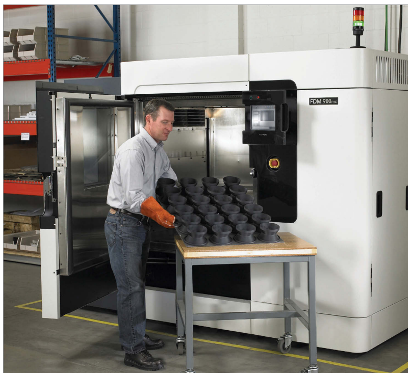
An engineer removes parts from the Stratasys Fortus 900mc machine, which was designed for direct digital manufacturing (DDM). Image courtesy of Stratasys
